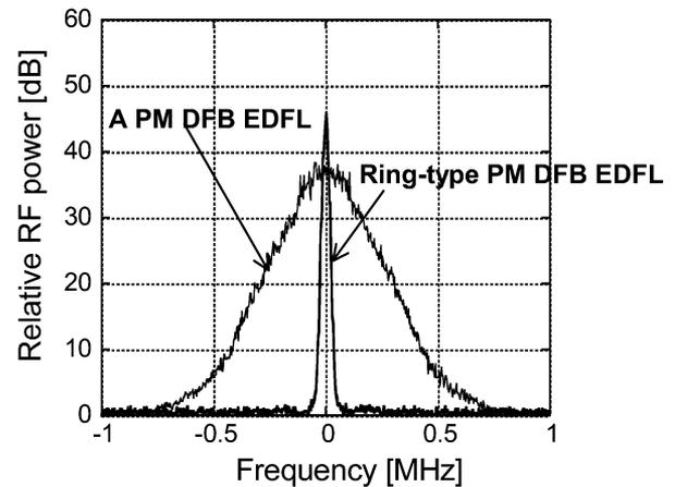
Fig. 4. Delayed self-heterodyne RF beat spectrum of conventional and 57-m ring-type PM  $\lambda/4$ -shifted DFB EDFL.
