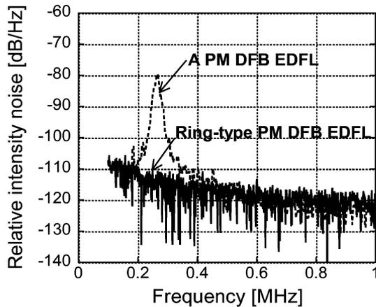
Fig. 5. RIN spectrum of conventional and 57-m ring-type PM  $\lambda/4$ -shifted DFB EDFL.
