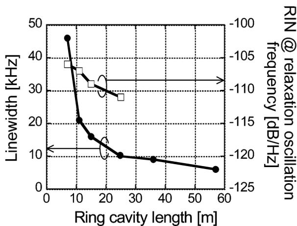
Fig. 6. Changes in the linewidth and RIN at relaxation oscillation frequency of ring-type PM  $\lambda/4$ -shifted DFB EDFL as a function of ring cavity length.
