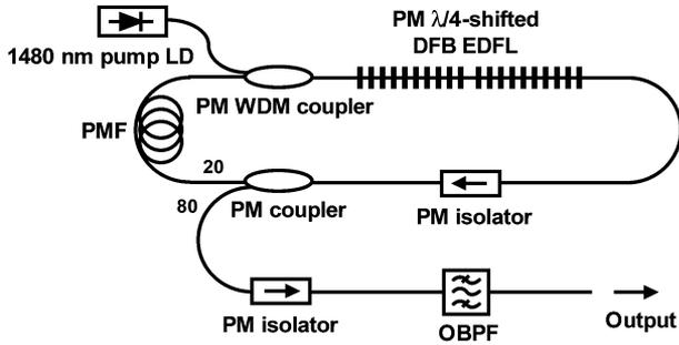
Fig. 2. Configuration of a ring-type PM  $\lambda/4$ -shifted DFB EDFL.
