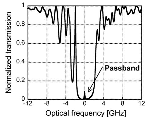
Fig. 1. Measured transmission spectrum of the  $\lambda/4$ -shifted FBG. (40-MHz resolution.)
