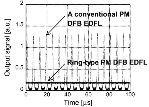
Fig. 3. Changes in the output signals of conventional and ring-type PM  $\lambda/4$ -shifted DFB EDFL.
